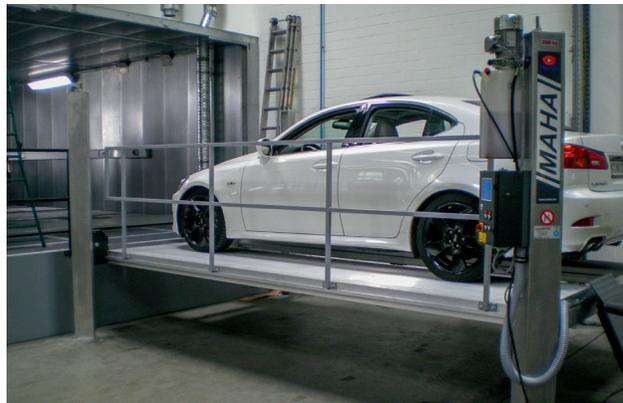
The Cologne-based company Toyota Motorsport GmbH, a test and development company specialised in advanced technology, required a dynamometer for its vehicles. The MSR 1000 from MAHA which was chosen for this purpose is usually installed in-ground to reduce the drive-on height.
