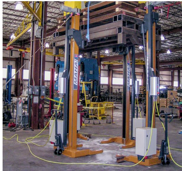
This central computer has a display through which the exact lifting height can be entered. The closer the support points converge to the mirror, the slower they become, until they eventually approach a pace of 1/10 mm. This is to avoid any juddering caused by sudden lifting, and the extremely expensive and fragile mirrors can therefore be lowered to the hall floor safely.
