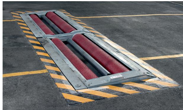
challenge of producing a brake tester specially adjusted to suit the vehicles' colossal dimensions while also being suitable for inspecting vehicles with hydrostatic drive motors. In the course of the project, the track width was therefore increased for the client while the roller length of the special test bench was expanded to 1,900 mm (the standard dimension being 1,150 mm).
