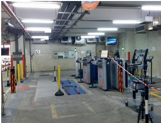
VICOM LTD commissioned MAHA Singapore to install two adjacent test lanes for motorcycles. As the test centre serves on average over 150 customers per day, a single test lane was not sufficient.
