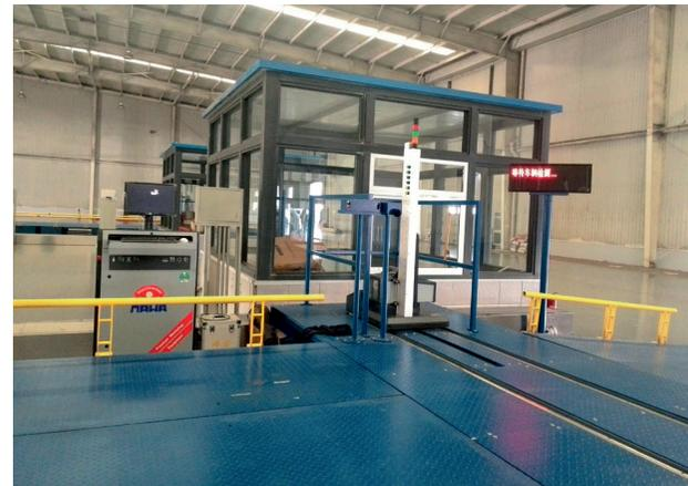
lane was installed for that very purpose. It contains the following six pieces of test equipment: the MGT 5 and MDO 2 emission testers, the MINC I side slip tester, the IW 2 EUROSYSYSTEM 4WD brake tester, the LITE 3 headlight tester and the FPS 2700 roller function tester.
