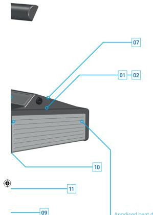
Anodised heat deflection sheet to prevent overheating as a result of direct sunlight even without use of the device covering hood.
