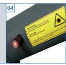
The unit is aligned with the vehicle by means of a mirror or, optionally, by using the laser pointer.
