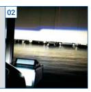
Pronounced blue fringing in the area of the cut-off line is reliably evaluated by the integrated control electronics.
