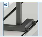
A rechargeable battery integrated into the base of the unit supplies the MLT 3000 with power for an entire working day and ensures a stable stand thanks to the low centre of gravity.
