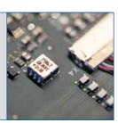
The electronic levelling system compensates for unevenness in the set-up area and is thus an absolute highlight of the MLT 3000. A deviation of only a few millimeters already results in an incorrect assessment of the measurement results. The deviations detected by the position sensor are automatically compensated by the MLT 3000 software, thus avoiding incorrect measurements.
