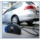
Diagnostic interface for testing the engine, safety and comfort electronics (OBD).
