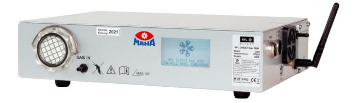
4-gas and 5-gas measurement device. Module for measuring petrol emissions: HC, CO, CO $_2$ , O $_2$  and lambda. Optional extension to include NO $_x$ .
