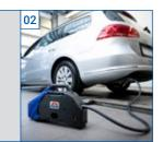
Diagnostic interface for testing the engine, safety and comfort electronics (OBD).
