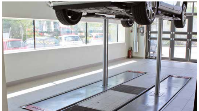
Vehicle lifted by the sill
