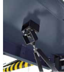
Fastening system and locking device for runway support.
