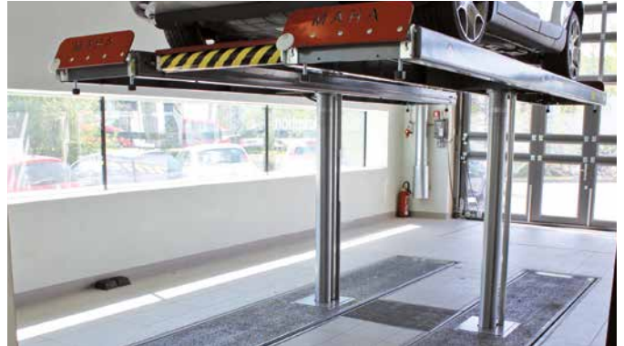
Vehicle lifted by the wheels
