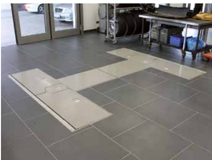
Fully covered swing arm support, traversable with 2 t wheel load
