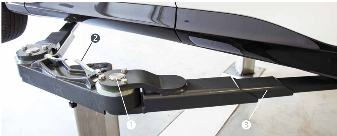
Swing arm support with tool tray.
