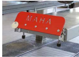
Automatic folding roll-off protection
