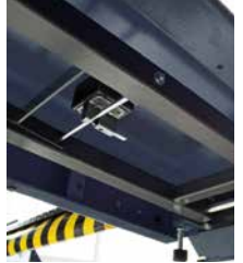
Fastening system and locking device for runway support.
