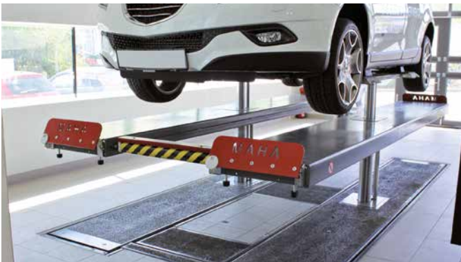
Setting of wheel-free jack or wheel inspection from the side
