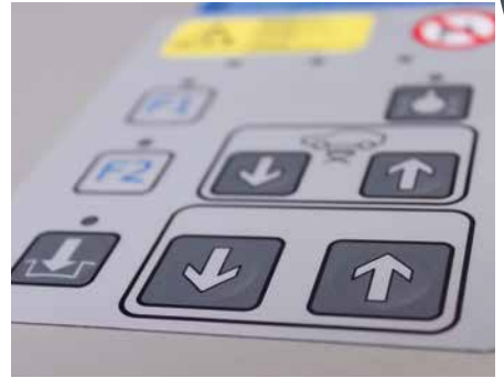
Membrane keypad with easy-to-operate micro-switches
