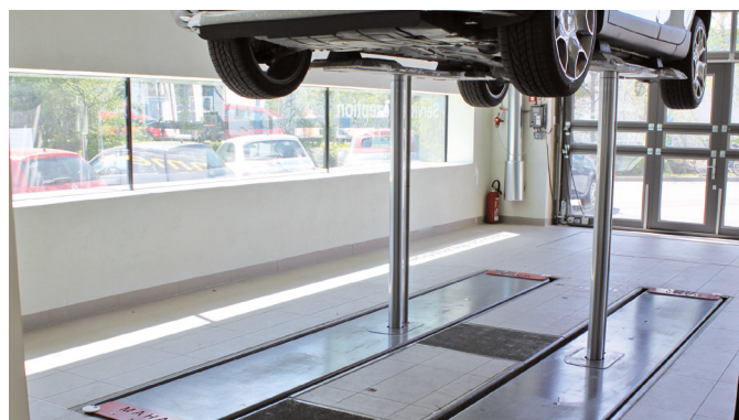
Vehicle lifted by the sill
