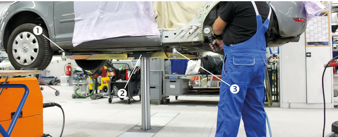
Safe and smooth locking of support arms using a detent mechanism.
