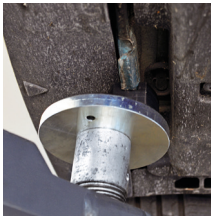
Very flat extension for easy access to car lifting points.
