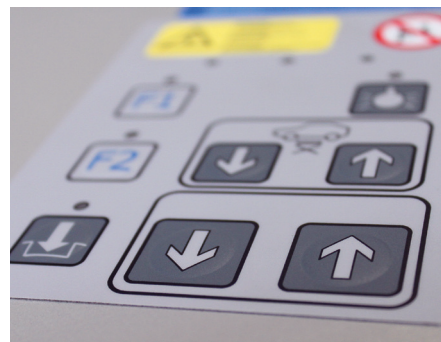
Membrane keypad with easy-to-operate micro-switches
