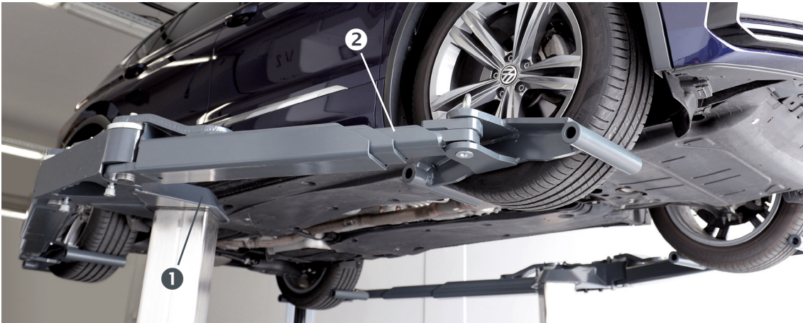
Safe support of vehicles by means of mobile column lift support also for 4.5 t lifts.
