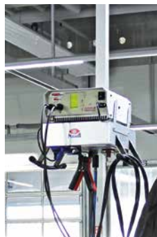
E-BOX version for DEUTRONIK, GYS-FLASH and ELTEK charging computer.
