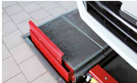
The floor compensation under the runway is a second ground surface, which levels off the surface below the lift.
