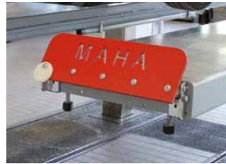
Automatic folding roll-off protection
