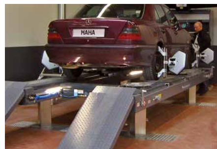
Highly accurate as a wheel alignment lift
