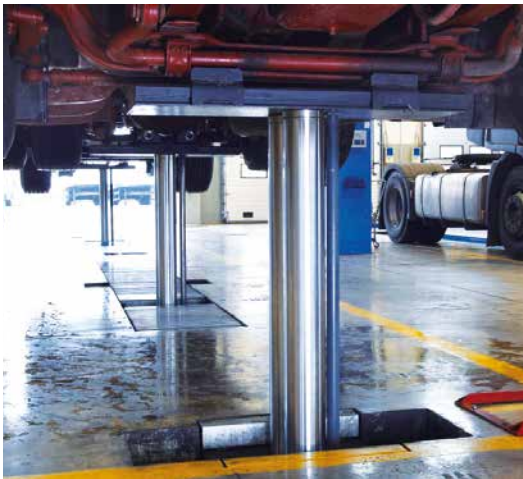
All MAHA TRUCKLIFT systems have synchronization control based on DIN EN 1493.
