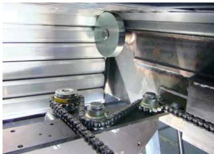
Secure chain guidance for exact positioning of the lifting unit
