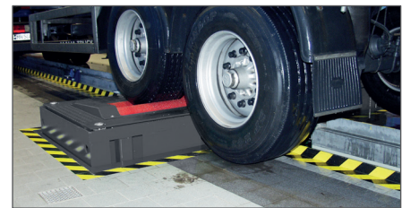
Roller set lifting Hydraulic roller set lifting for axle load displacement on the axle being tested.
