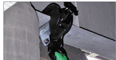
Fastening clips For fastening the belt to the vehicle frame.
