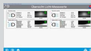
Light test Digital determination of the headlight setting by means of a CMOS camera.
