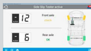
Side slip test Clear display of the directional stability of the vehicle axles.
