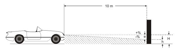
Angle of inclination of light-dark limit against the test surface.
