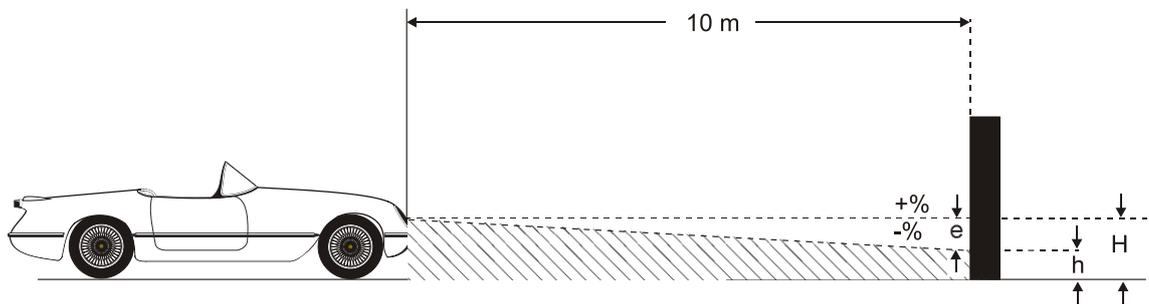
Angle of inclination of light-dark limit against the test surface.
