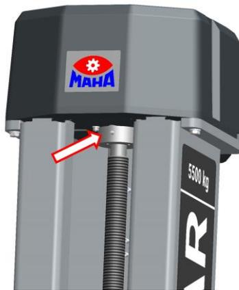
Lubricate the upper spindle bearing at least once a year. Lower the lifting carriage to bottom position; loosen the spindle cover at the head plate and remove it. Then lubricate the spindle bearing with multipurpose grease through the lubrication nipple. For lubrication points, see section "Maintenance > Lubrication > Lubrication Points and Lubricants".
