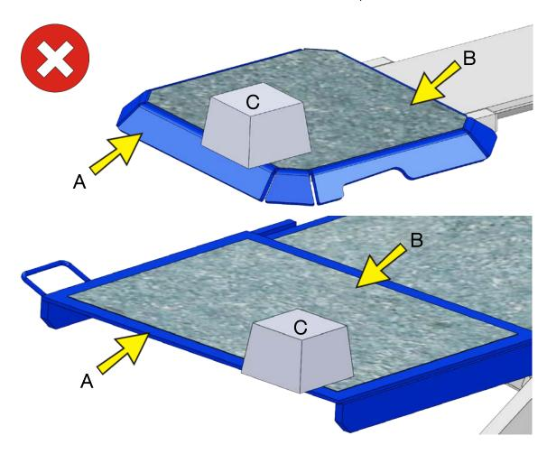
Diagonal positioning is permissible only with granulate coated surfaces (a). If knobbly pads are used, these must mesh with the support blocks (b).
