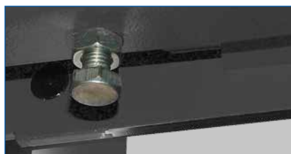
Transverse beams adjustable to baseplate in fully lowered position.
