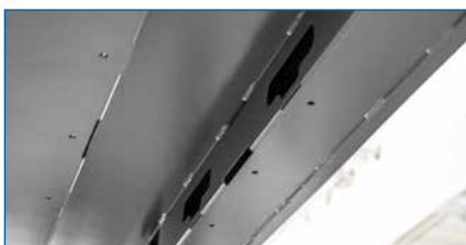
Additional reinforcement plates within the runways welded for high torsional and bending stiffness.
