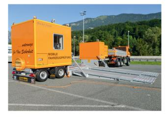
The MBT 7250 EUROSYSTEM roller brake tester and the LMS 20/2 axle play tester with crawler chassis are used.
