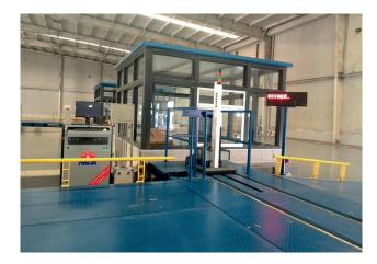
lane was installed for that very purpose. It contains the following six pieces of test equipment: the MGT 5 and MDO 2 emission testers, the MINC I side slip tester, the IW 2 EUROSYSTEM 4WD brake tester, the LITE 3 headlight tester and the FPS 2700 roller function tester.
