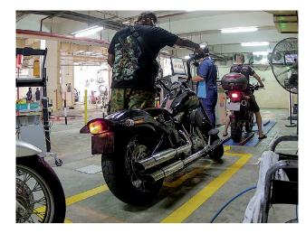
time, as checks were to take place in parallel. A complete function test includes a visual inspection as well as an inspection of the noise level, the emissions, the head-lights, the brakes and the side slip.
