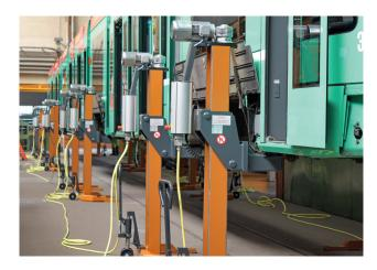
This is why 16 mobile wheel engaging column lifts were installed by MAHA, rather than the usual 12. The challenge was to align all the columns with extreme accuracy, since the synchronous running of the wheel engaging systems has to be ensured.
