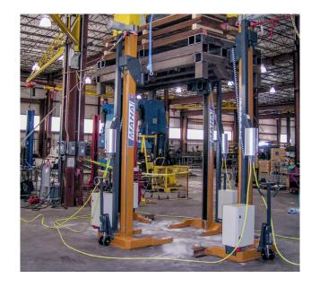
This central computer has a display through which the exact lifting height can be entered. The closer the support points converge to the mirror, the slower they become, until they eventually approach a pace of 1/10 mm. This is to avoid any juddering caused by sudden lifting, and the extremely expensive and fragile mirrors can therefore be lowered to the hall floor safely.
