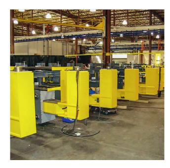
During the production process, MAHA USA created a special test station in which – before the lift was delivered to New York – each of the individual lifting segments were tested at full load. The lifting system and the electromechanical rotary disc were successfully installed in early 2009.
