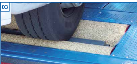
The test-lane-compatible roller brake tester MBT 7000 is designed for the brake testing of vehicles with axle loads up to 18.0 t and is ideal for vehicles diagnostics in situations of high vehicle throughput.
