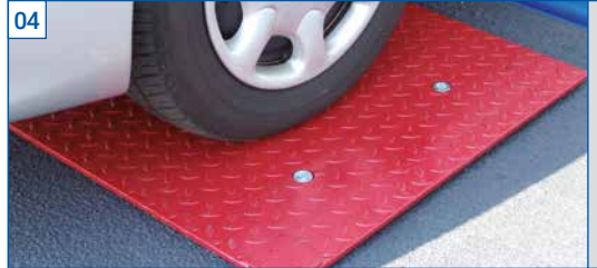
The axle play tester LMS 20.0 is intended for the reliable determination of defects and wear on steering parts, wheel bearings, shock absorbers and suspension by lateral and longitudinal movement of the test plates in opposite directions. An automatic mode as well as other different operating modes ensure the uncomplicated operability of the LMS 20.0.
