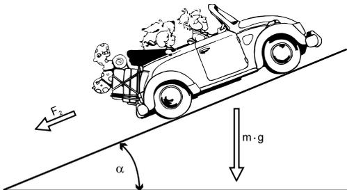
Calculation of the traction  $F_{st}$
