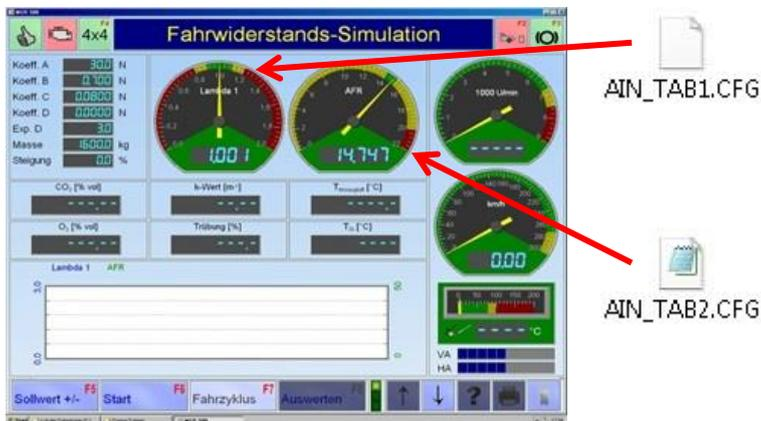
Additional option: Lambda dial. Lambda value can be displayed instead of engine rpm.
